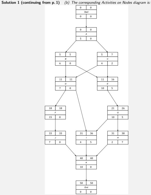
$\begin{bmatrix} 0 & | & 0 \end{bmatrix}$  (c) Activities on the critical path, A, B, D, F, J, and K, have float of 0. Activity C has float of 2,
